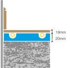
Heat output of up to 80watts/m²
