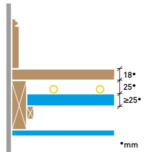
Heat output of up to 100watts/m<sup>2</sup>
