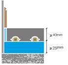
Heat output of up to 120watts/m<sup>2</sup>
