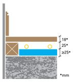
Heat output of up to 100watts/m²
